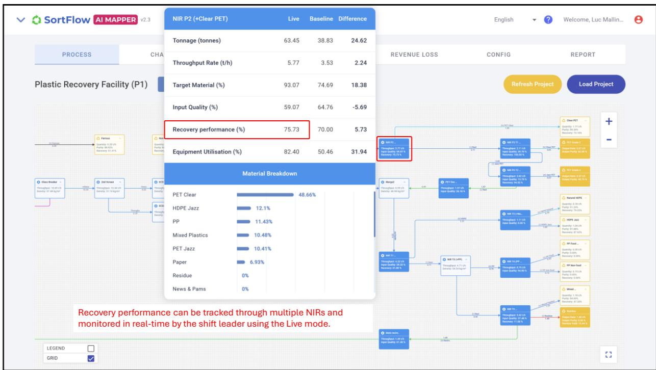
Recovery performance can be tracked through multiple NIRs and monitored in real-time by the shift leader using the Live mode.
