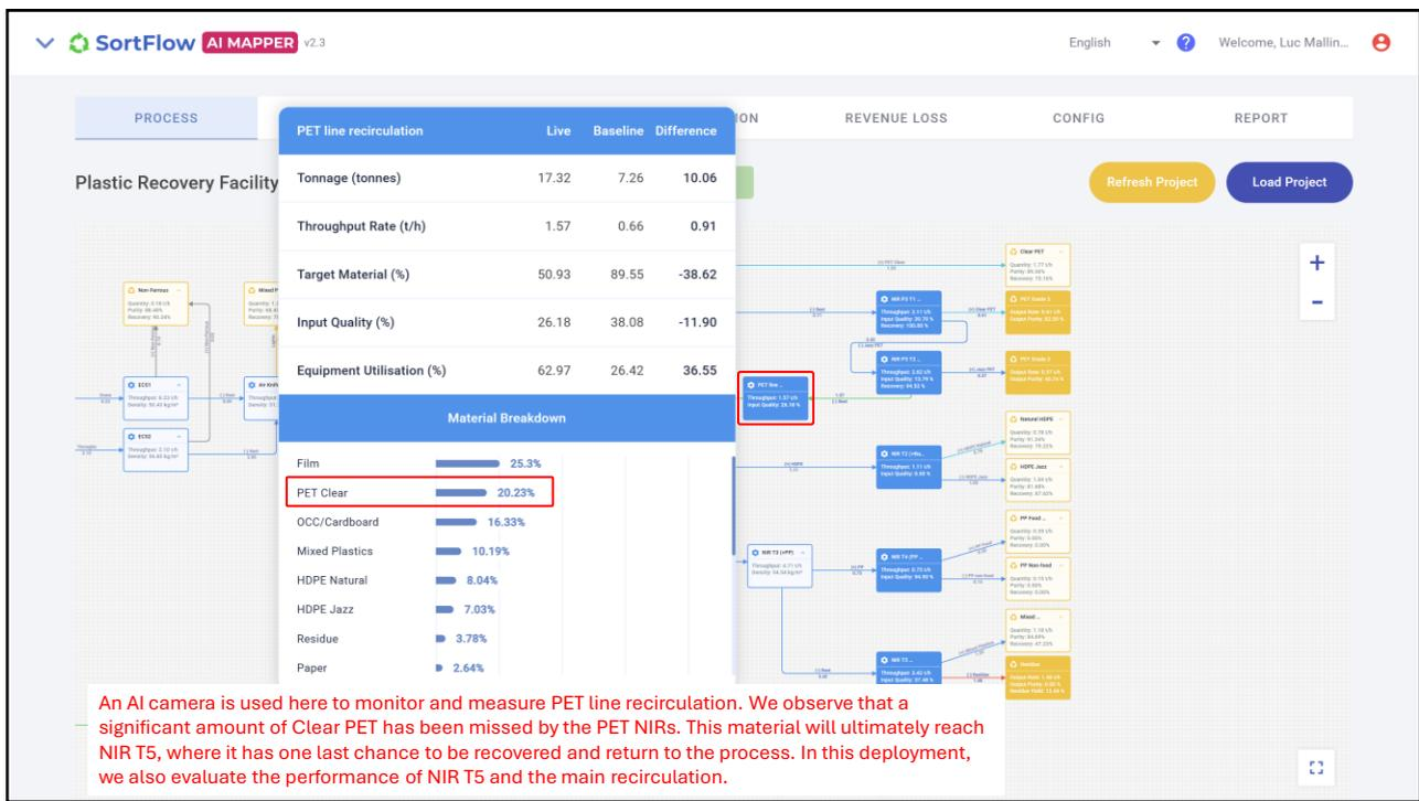
An AI camera is used here to monitor and measure PET line recirculation. We observe that a significant amount of Clear PET has been missed by the PET NIRs. This material will ultimately reach NIR T5, where it has one last chance to be recovered and return to the process. In this deployment, we also evaluate the performance of NIR T5 and the main recirculation.
